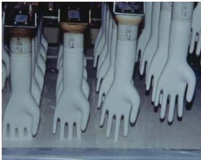
Glove formers being dipped into the liquid glove solution.
